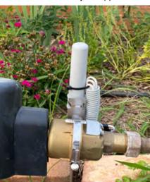
Clip on device - These attach to existing meters which are working fine and are not due for replacement in the coming years
